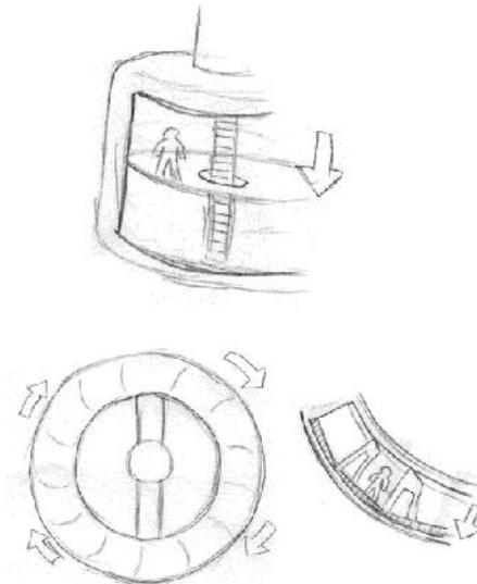
**Image 2: concepts for torus and pendulum centrifuge operation**
